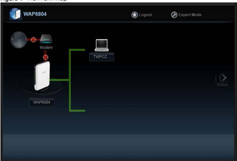
The line connecting the WAP6804 to the gateway becomes green when the WAP6804 is able to ping the gateway. It becomes red when the ping initiating from the WAP6804 does not get a response from the gateway. The same rule applies to the line connecting the gateway to the Internet.
