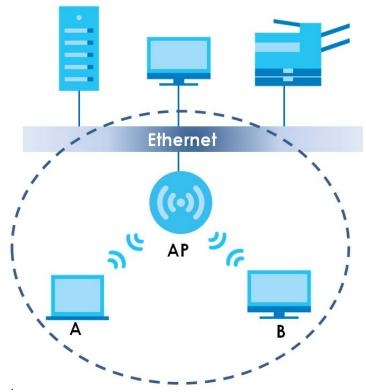
The wireless network is the part in the blue circle. In this wireless network, devices **A** and **B** are called wireless clients. The wireless clients use the access point (**AP**) to interact with other devices (such as the printer) or with the Internet. Your WAP6804 is the AP in the above example.
