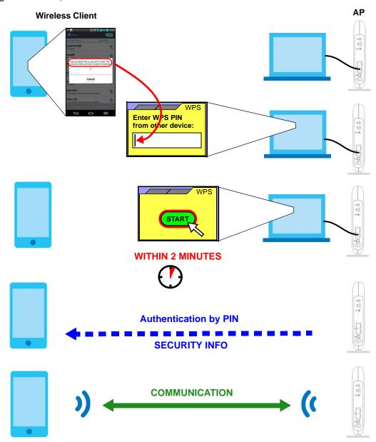
Figure 22 Example WPS Process: PIN Method
